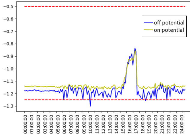
Fig. 1. Potential curve under HVDC interference
