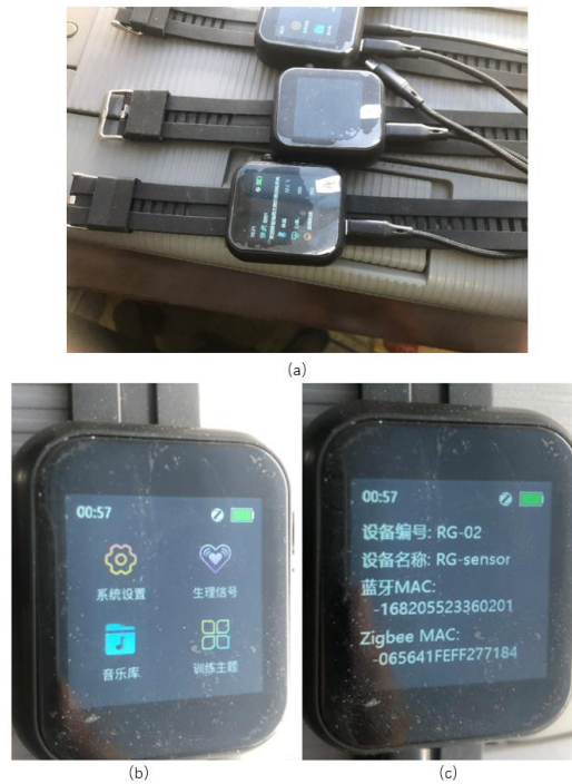
Fig. 1. Watch style display, (a) wearable watch (b) watch page function (c) system setting page in watch page.
